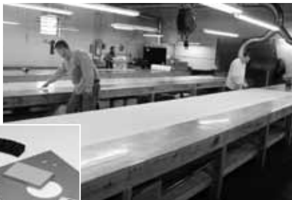
Dean Swisher (left) and Mike Sisco (right) apply custom adhesives in Stockwell’s lamination department.
